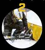
Attach the winch cable to the plow using a guiding hook/roller.
